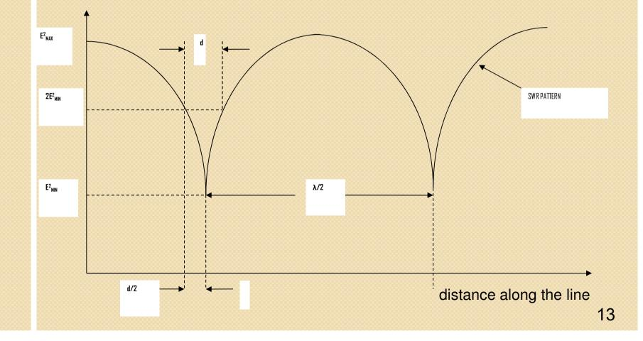
The detector output (proportional to field strength squared) is plotted against position. The probe is moved along the line to find the minimum value of signal.
