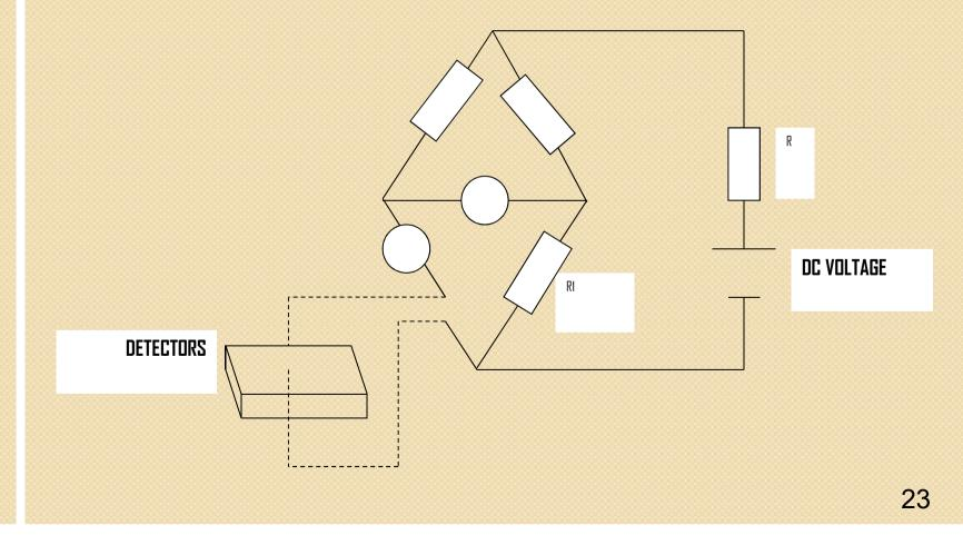
• With no power to the detector that contains the sensor element, the sensor-line RI is adjusted to zero reading through the meter MI and the bridge circuit is balanced.
